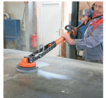
Cleaning shuttering segments in upright position
